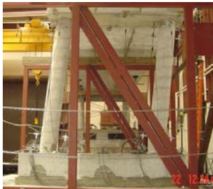
Figure 5. Middle bent before (left) and after (right) straightening.
