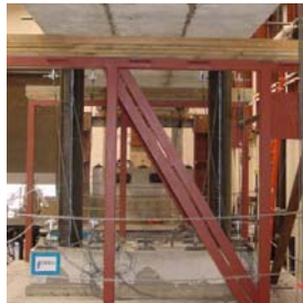
Figure 5. Middle bent before (left) and after (right) straightening.
