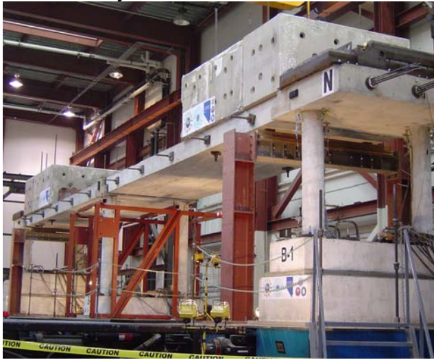
Figure 1. Two-span bridge test set up
